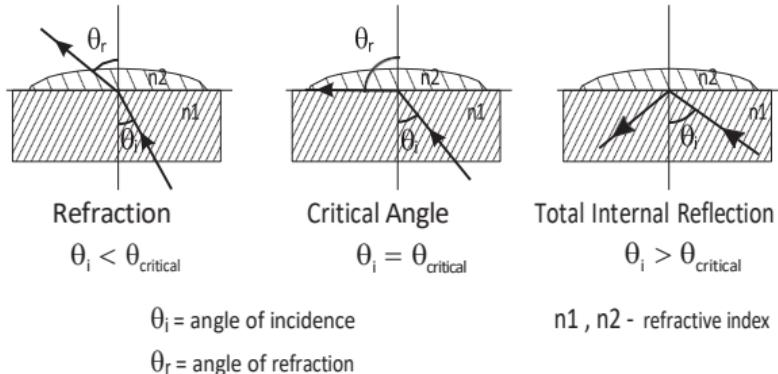
In the **MA872**, light from an LED passes through a prism in contact with the sample. An image sensor determines the critical angle at which the light is no longer refracted through the sample. The **MA872** automatically applies temperature compensation to the measurement and converts the refractive index of the sample to Fructose concentration in units of percent (by weight).
