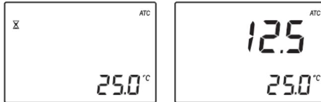
**Note:** The ATC tag blinks and automatic temperature compensation is disabled if the temperature exceeds the 10-40 °C / 50-104 °F range.
