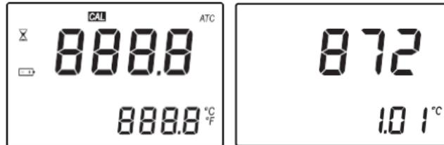
2. While continuing to hold the **ON/OFF** key, press the **ZERO** key. The temperature unit will change from °C to °F or vice versa.
