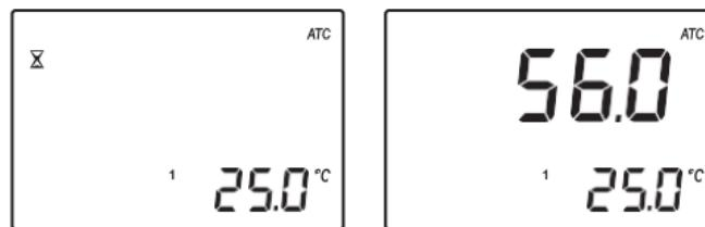
**Note:** The last measurement value will be displayed until the next sample is measured or the instrument is turned off. Temperature will be continuously updated.
